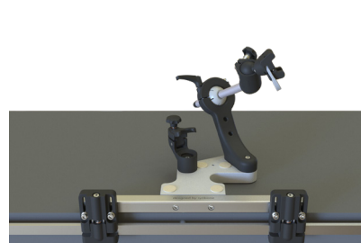
To use the ROB Knee Holder System with right-sided knee models the Base Plate has to be flipped by 180°
